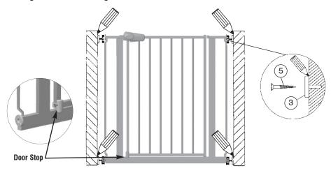
Fitting the Gate: Do not remove the gate door securing tie until the gate has been fitted.
