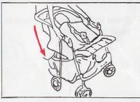
B. Pull up folding latches at sides of handle. Fold handle down.
