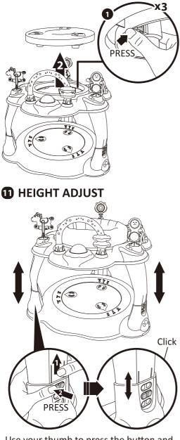
Use your thumb to press the button and press down until a "Click" sound. Press the button to adjust 3 section height.
