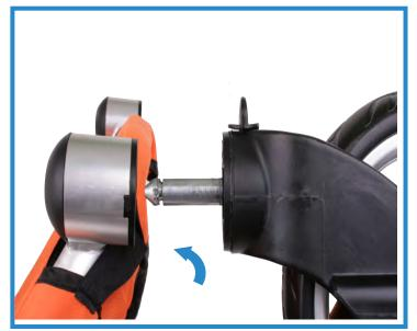
To **assemble the front wheels**, place each front wheel and insert it into each of the wheel mouldings.
