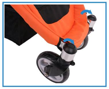
To **remove the front wheels**, press the buttons located on the top of the wheels mouldings then pull down on wheel to remove it. Repeat for both sides.
