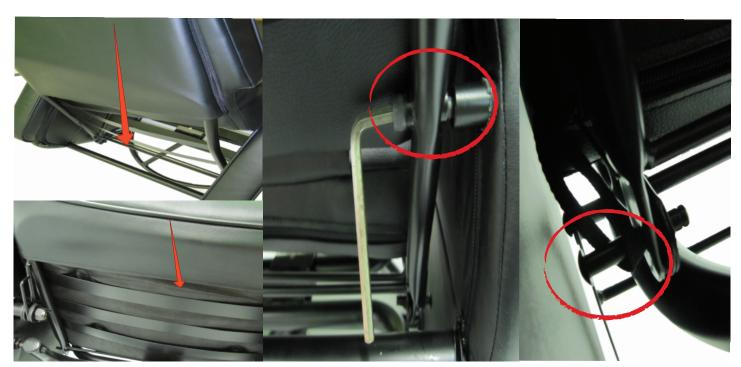
Place the cushion (3) over the backrest and the bottom seat. They should be placed over the bars as shown.
