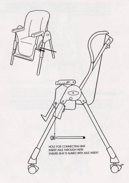
III. HOOK THE SEAT ONTO THE SEAT SUPPORT LOCATED ON TOP OF FRAME.
