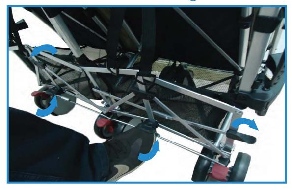
To Fold the stroller, Kick or push up the 2 middle latches on the rear axel, then pull the side levers downwards
