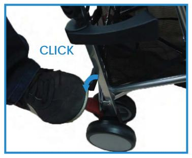
To lock the rear wheels, press down on rear right red brake pedal to lock the brakes. Check that the brakes have been engaged by pushing the stroller forward.
