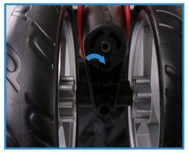
To remove the front wheel, press the button located on the bottom of the wheels moulding then pull down on wheel to remove it.
