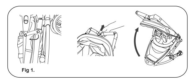
1. Unfold the frame - remove the locking latch. Grasp both handles and lift up quickly to open frame and press down the handles until you hear clicks. Pull up the upper Lock as shown in Fig. 1
