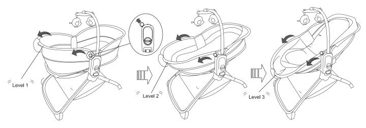
The angle can be adjusted by pulling the adjusting device
