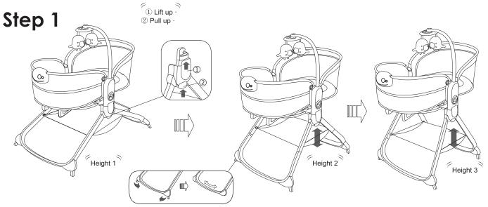
The Height can be adjusted by pulling the adjusting device
