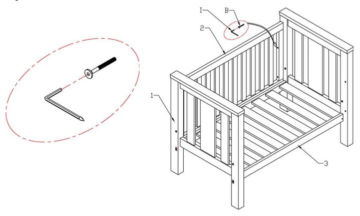
**Step 4** Attaching the Screw for the dropside
