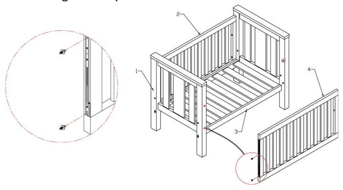
$_{Step\ 6}$  Tightening the screw for the dropside
